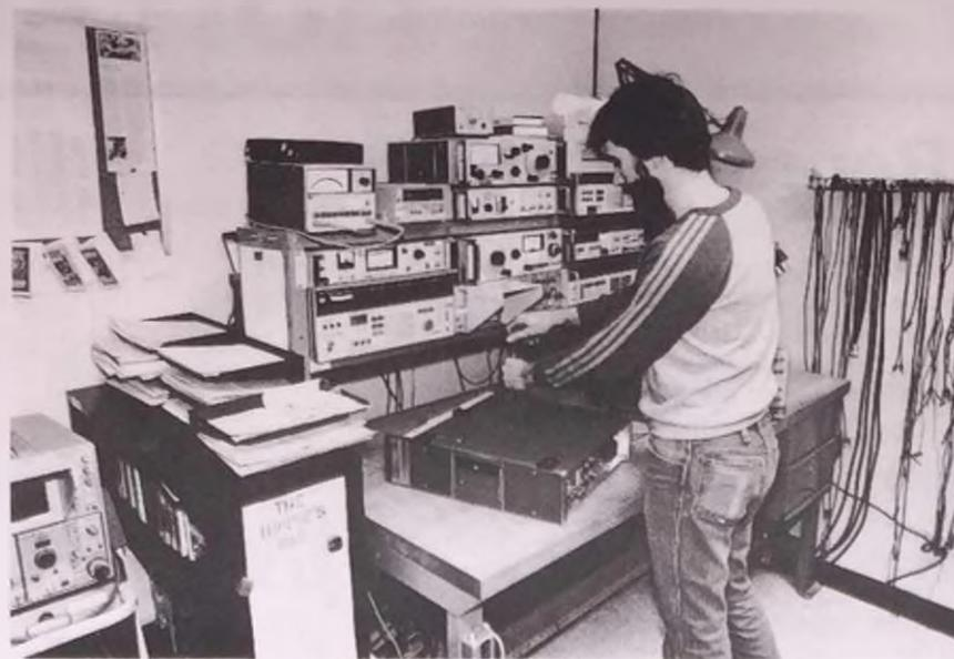
Bob Reinert, a metrology technician in the RF (radio frequency) lab, works with precision DC equipment in making his high-accuracy measurements. Most of the equipment he calibrates is used by design engineering. In checking radio frequencies, Bob compares them to a standard frequency which is radio broadcast from the NBS office in Ft. Collins.
