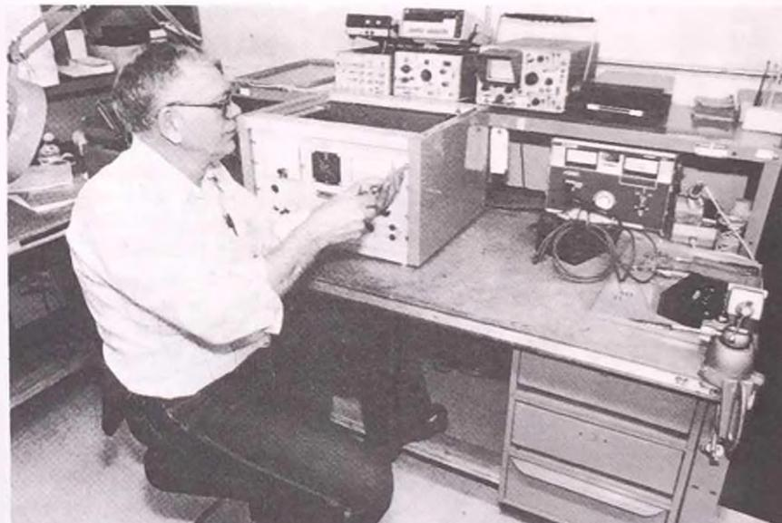
Wilbur Petty, a metrology technician III, here deals with an AC insulation tester, used to check for breakdowns in insulation in STC's end products. An amateur astronomer, Wilbur makes his own telescopes in his time off.
