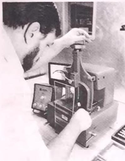
The gage lab within the metrology lab has stringent temperature and humidity controls, plus a positive pressure environment, to minimize physical variations and dust. Here Charlie Steffens, a quality engineer, uses the gage block comparator to compare gage blocks (the standards for linear measurements) against a master set obtained from the National Bureau of Standards. The equipment can measure differences in the blocks of plus or minus a millionth of an inch.
