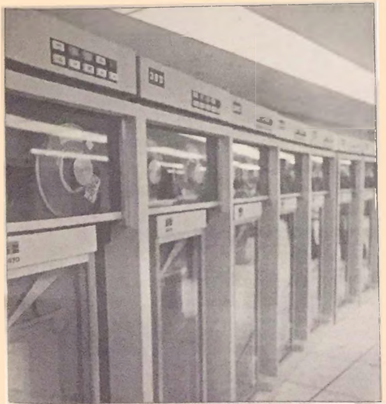
COURTESY STORAGE TECHNOLOGY CORP Storage Technology's first product, recorded for this picture in 1970, was the 2470 computer tape drive.
