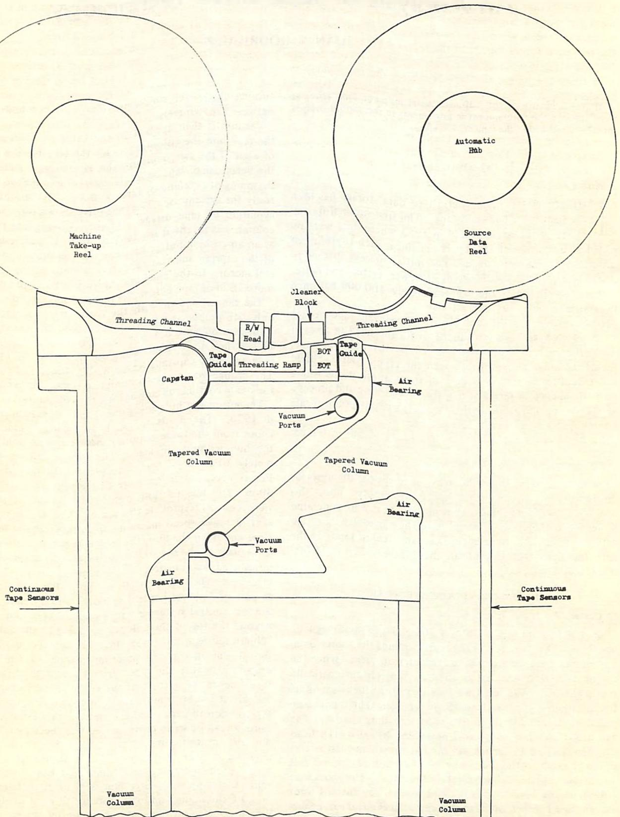
Fig. 1. Typical tape path area of magnetic tape unit.
