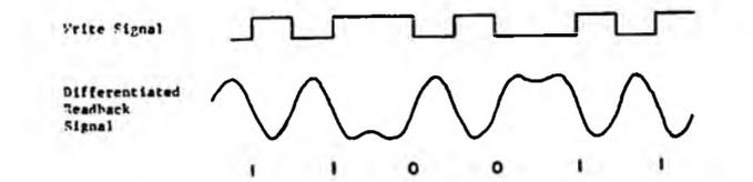
Fig. 3. Phase-encoded recording.
