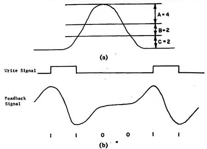
Fig. 2. (a) Isolated pulse showing write detection band. (b) NRZI recording.
