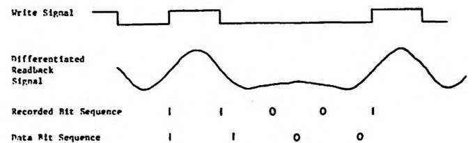
Fig. 4. Group-coded recording.
