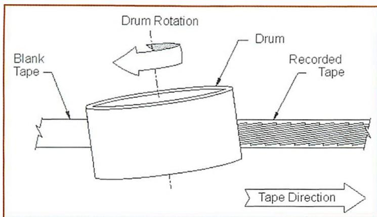
**Fig 3** The head-tape interface consists of a drum containing the read and write heads rotating at a fixed speed of 4,345rpm. The axis of the drum's rotation is perpendicular to the path of the tape. As the drum rotates, the heads move from the lower to the upper edge of the tape.
